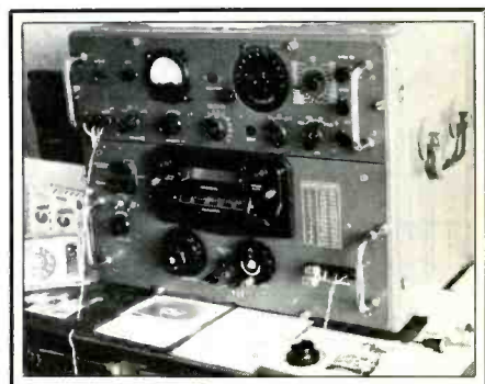
R-250 vintage military receiver—the most popular one among Soviet DX'ers (still no BFO circuit and an analogue scale).
